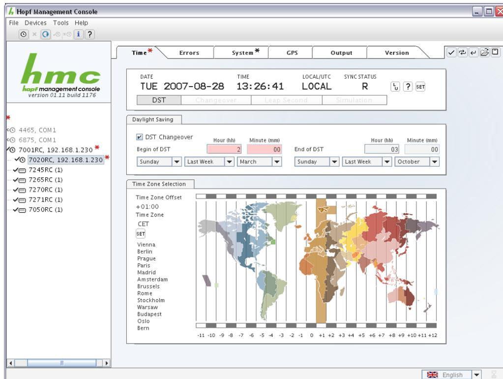
An example of an invalid input in the tab area *Time*. The *System* tab holds a black asterisk, indicating a value change. The device tree only shows a red asterisk which implies a value change anyway.
