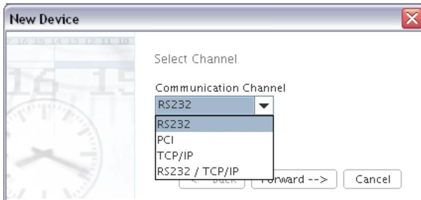
First, the Communication Channel to the device to be opened has to be defined. This will be either a serial connection (*RS232*), or a connection to a device that is directly integrated with the computer, e.g. a PCI board (*PCI*), or a device connected via the Internet or a local network (*TCP/IP* or *RS232 / TCP/IP*).
