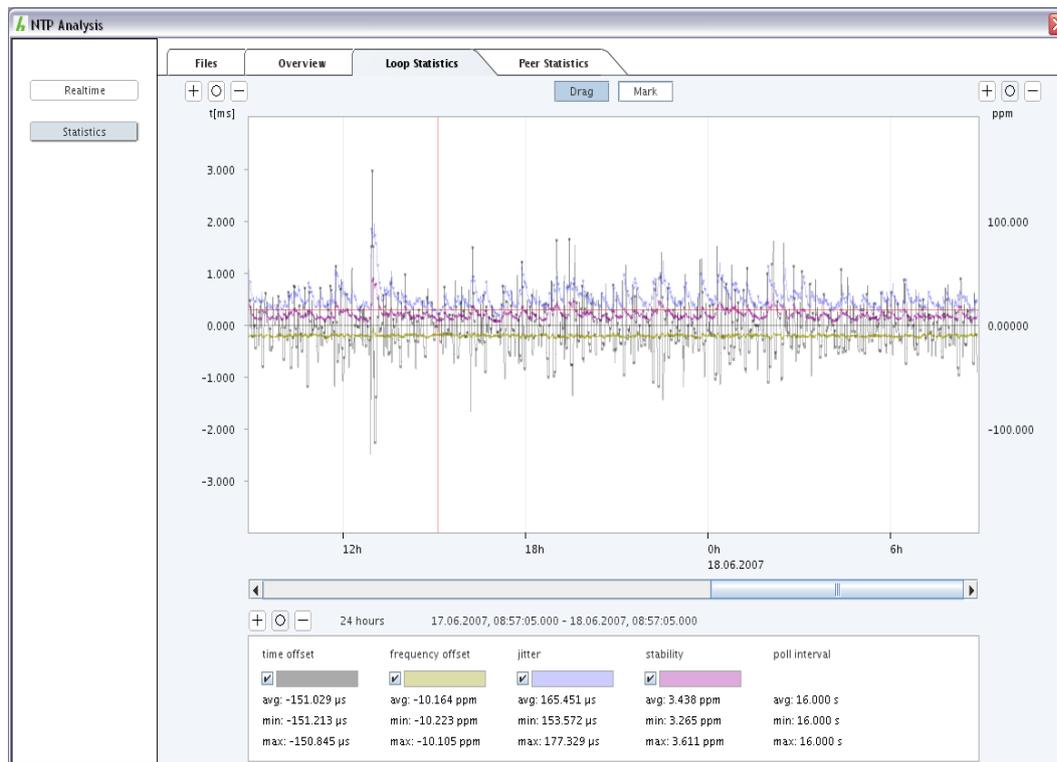
Loopstat files are shown in the *Loop Statistics* area. For the left scale (time, for time offset and jitter), the right scale (ppm for frequency offset and stability), as well as the bottom time scale, the buttons ,  and  allow zooming in, resetting the zoom factor, and zooming out.
