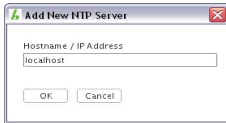
After entering a host name or IP-Address and confirming with the OK-Button a new Tab is added to the NTP panel.
