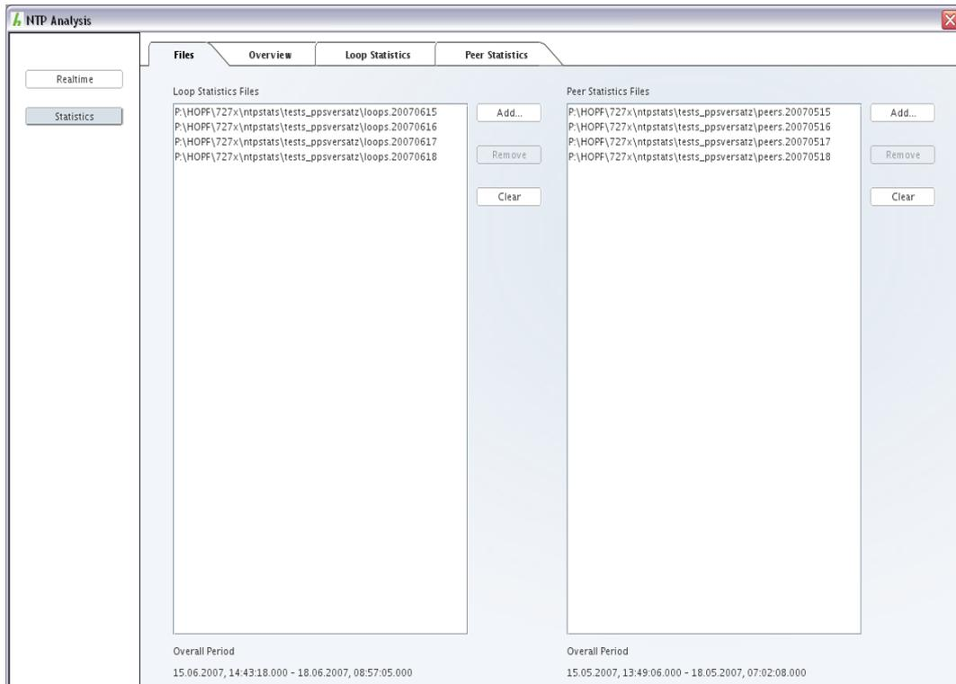
In the *Files* area, one or more loopstat and peerstat files may be added, and removed again.
