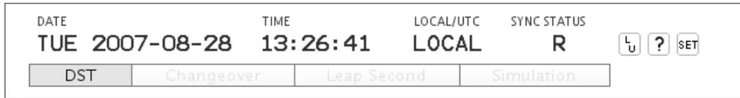
In this case, a time and date local to the selected time zone (see below) is shown. Automatic daylight saving time changeover is active, thus the clock, at the given date in August, is in daylight saving time mode. This fact is shown below the date / time view. The other possible state indicators are:
