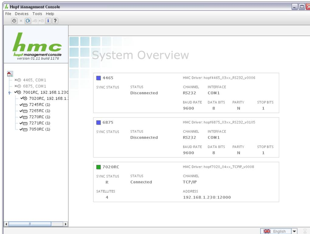
The system overview panel is reached by selecting the main element in the device tree. To return to the start screen, a single click in the HMC logo area above the device tree is necessary.
