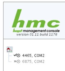
It is possible to hold in the tree several disconnected devices that are all configured for the same serial port of the computer (as shown in this example a **hopf** 4465 and a **hopf** 6875 on port COM2). But of course, only one connected device is possible for a given port at a time. All devices in the device tree will sustain after restarting the HMC. Previously connected devices will be not be automatically reconnected.
