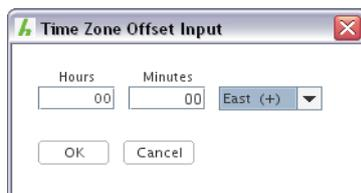
A time zone can be specified manually too (up to minute precision). For this purpose, the button **SET** will open a dialog allowing to input an offset in direction, hours and minutes.
