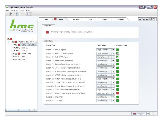
In the 7020RC / 7050RC's configuration area there is a tab *Errors* which allows the definition of filters for all possible error states of the 7001RC system. For every error, there are four priority settings: *High*, *Low*, *High Ignored*, *Low Ignored*.
