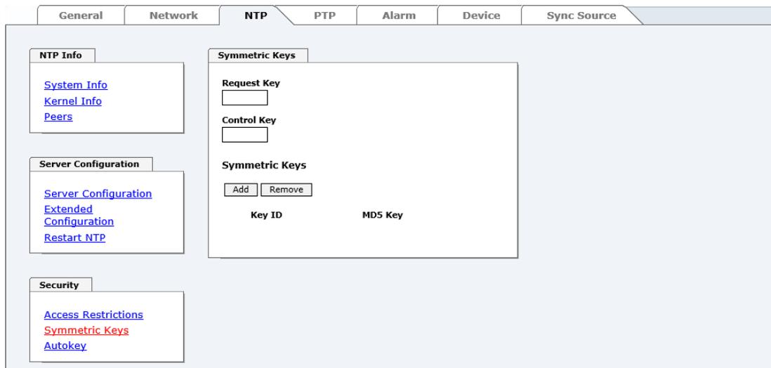
The screenshot shows the NTP configuration web interface. The top navigation bar includes tabs for General, Network, NTP (selected), PTP, Alarm, Device, and Sync Source. The main content area is divided into three sections:
