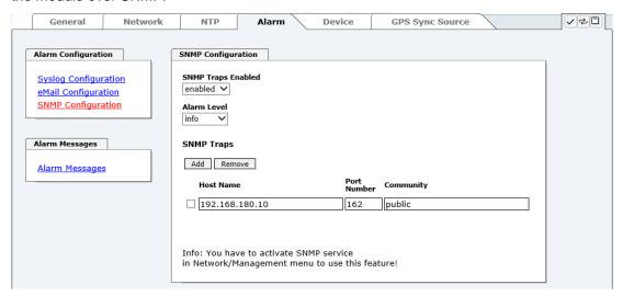
SNMP traps are sent to the configured hosts over the network. It should be noted that these are based on UDP and therefore it is not certain that they will reach the configured host!
