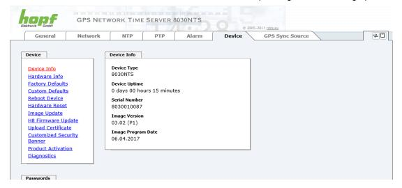
This tab provides the basic information about the hardware of Module 8030NTS as well as software/firmware. Password administration and the update services for the module are also made accessible via this website. The complete download zone is also a component of this site.
