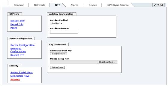
In order to enable Autokey v2 authentication, the "Autokey Enabled" option must be set to "enabled" and a password specified (may not be blank).
