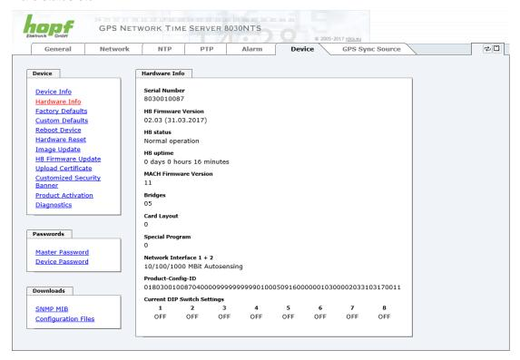
The display "Current DIP Switch Settings" is not applicable for this device.
