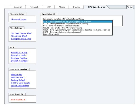
The output of the status optical coupler (on the front panel of the Time Server 8030NTS/GPS) can be configured by the use of this function.
