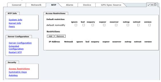
Restrictions are used in order to control access to the System's NTP service and these are regrettably the most misunderstood options of the NTP configuration.
