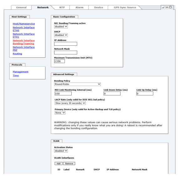
This function is used for the distribution of load as well as to increase fail-safety in computer networks.
