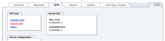
This screenshot shows a maximum kernel clock error of 6.500 msec (milliseconds). The estimated error value is 2 µs (microseconds).
