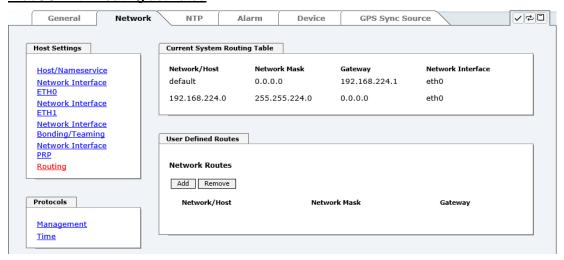
The image above shows every configured route of the base system routing table as well as the user's defined routes.
