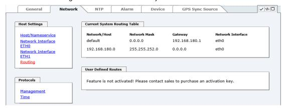
The gateway / gateway host need to be in the local sub-network range of the module in order to use the routes.
