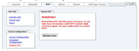
Restarting NTP services is the only possibility of making NTP changes effective without having to restart the entire Time Server 8030NTS/GPS. As can be seen from the warning message, the currently reachable stability and accuracy get lost caused by this restart.
