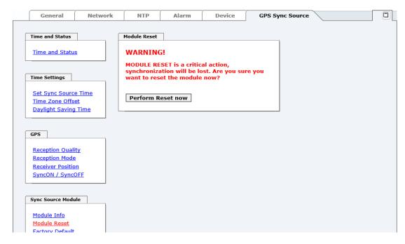
This function triggers a hardware reset of (just) the Sync Source (here Module 8024GPS).
