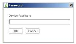
The Time Server 8030NTS/GPS is supplied with the default device password <device> on delivery. After entry click on the OK button to confirm.
