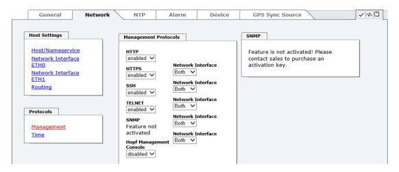
After an entry with **Apply** is made, the configured field is marked with a star ' \* '. This means that a value has been entered or changed but not yet been stored in the flash memory.
