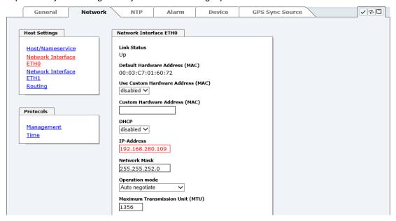
As illustrated in the above image, an invalid value (e.g. text where a number should be entered, IP address not within the range etc.) is identified by a red border when an attempt is made to accept these settings. It should be noted here that this is only a semantic check and not to test whether an entered IP address can be used on the own network or in the configuration! As long as an error message is displayed it is not possible to save the configuration in the flash memory.
