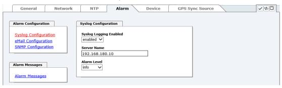
The alarm level designates the priority level of the messages to be transmitted and the level from which transmission should take place (see *Chapter 7.3.5.4 Alarm Messages*).
