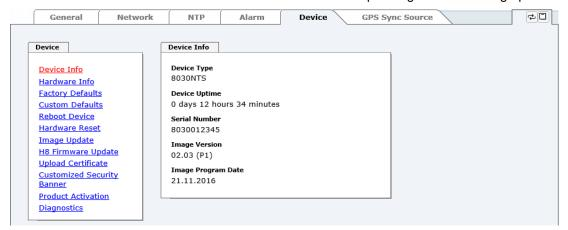
This tab provides the basic information about the hardware of Module 8030NTS as well as software/firmware. Password administration and the update services for the module are also made accessible via this website. The complete download zone is also a component of this site.
