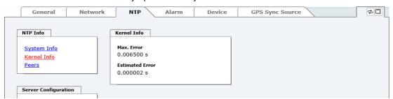
This screenshot shows a maximum kernel clock error of 6.500 msec (milliseconds). The estimated error value is 2 µs (microseconds).
