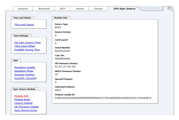
This tab indicates information about the hardware and software of the Module 8024GPS (Sync Source) implemented in the Time Server 8030NTS/GPS.
