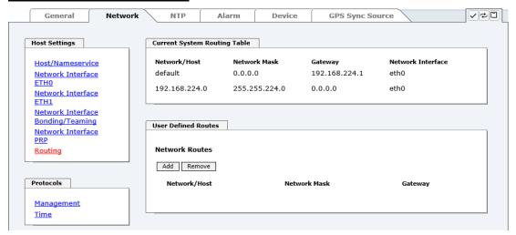
The image above shows every configured route of the base system routing table as well as the user's defined routes.
