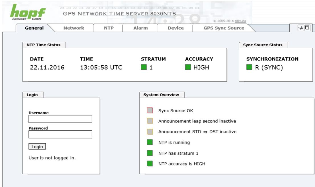
The screenshot displays the web interface for the hopf GPS NETWORK TIME SERVER 8030NTS. The interface is organized into several sections:
