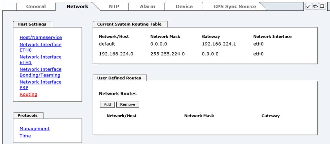
The screenshot shows the 'Network' configuration page with Routing enabled. The 'Current System Routing Table' contains the following entries:
