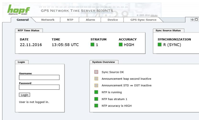
The screenshot shows the web interface for the hopf GPS NETWORK TIME SERVER 8030NTS. The 'General' tab is active, displaying the following information:
