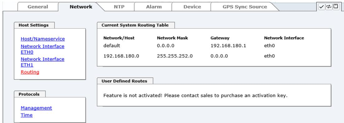
The screenshot shows the 'Network' configuration page. The 'Current System Routing Table' contains the following entries:
