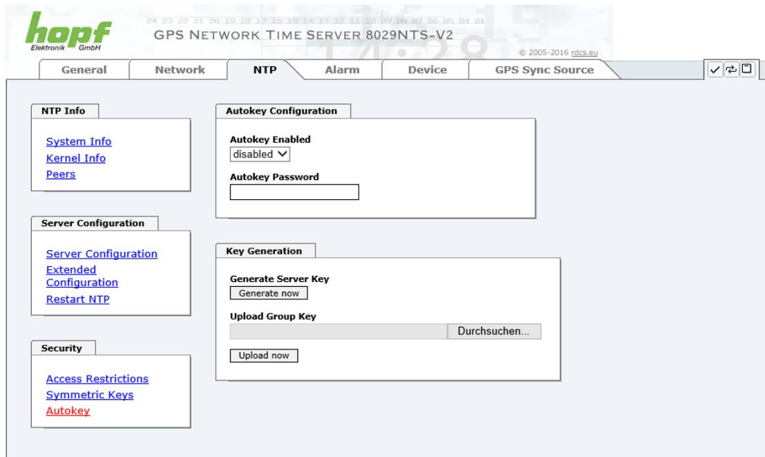
The screenshot shows the web interface for the GPS NETWORK TIME SERVER 8029NTS-V2. The 'NTP' tab is selected, and the 'Autokey Configuration' section is active. It includes a dropdown for 'Autokey Enabled' (currently set to 'disabled'), an 'Autokey Password' input field, and a 'Key Generation' section with 'Generate now' and 'Upload now' buttons. A search button 'Durchsuchen...' is also visible in the 'Upload Group Key' section.
