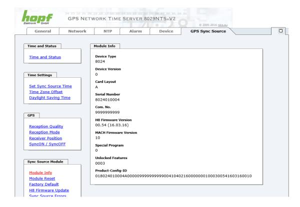
This tab indicates information about the hardware and software of the Module 8024GPS (Sync Source) implemented in the Time Server 8029NTS/GPS.
