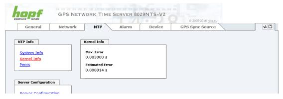
This screenshot shows a maximum kernel clock error of 3.000 msec (milliseconds). The estimated error value is 14 µs (microseconds).
