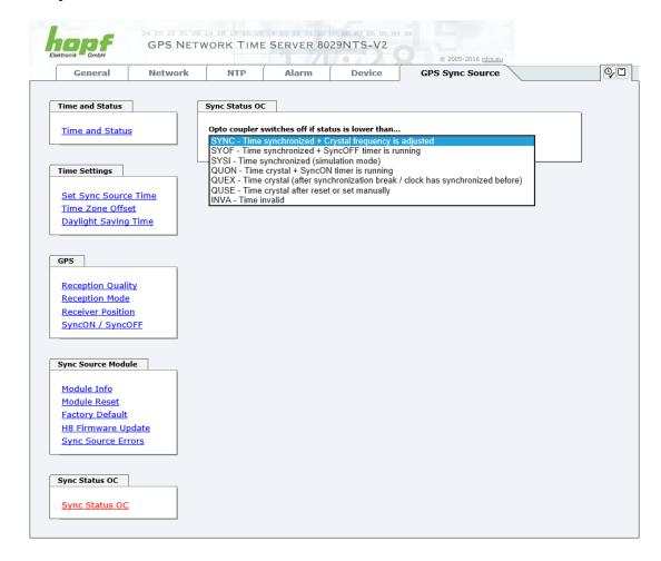
The output of the status optical coupler (on the front panel of the Time Server 8029NTS/GPS) can be configured by the use of this function.
