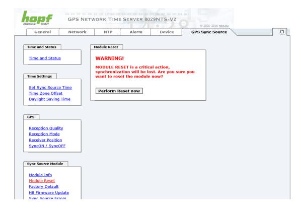
This function triggers a hardware reset of (just) the Sync Source (here Module 8024GPS).
