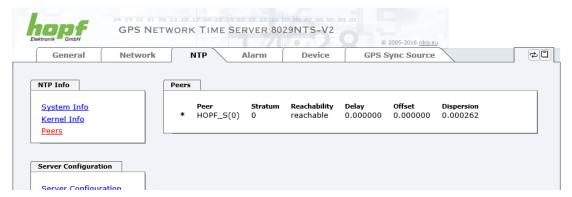
The first line displays the **hopf** - refclock ntp driver that gets the time information directly from the Sync Source.
