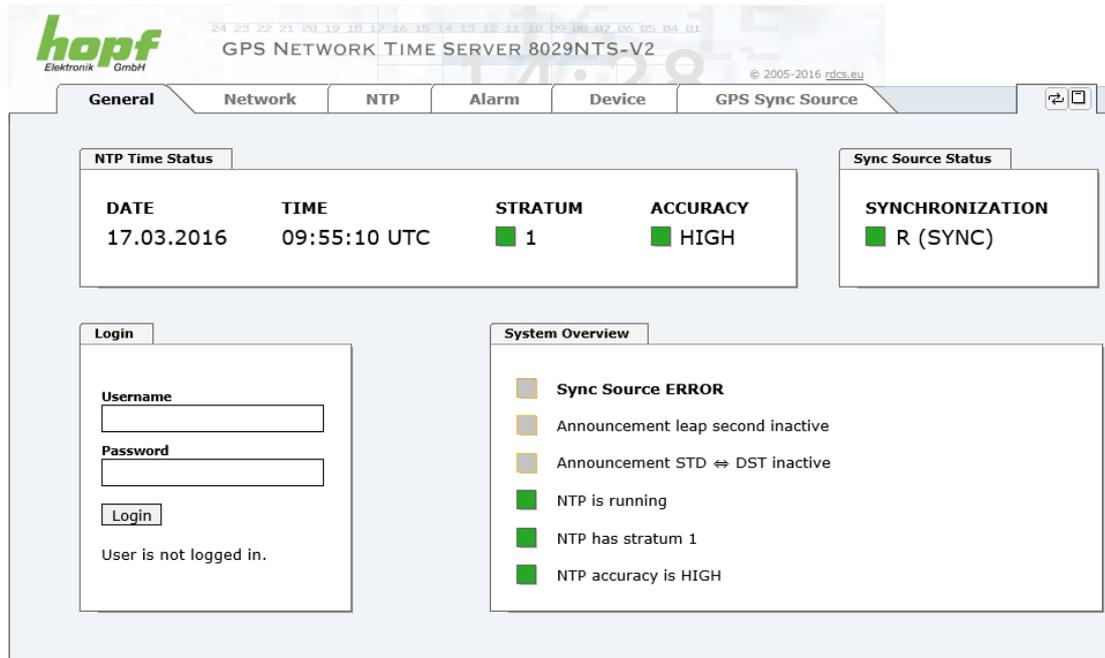
The screenshot displays the web interface for the hopf GPS NETWORK TIME SERVER 8029NTS-V2. The interface includes a navigation menu with tabs for General, Network, NTP, Alarm, Device, and GPS Sync Source. The main content area is divided into several sections:
