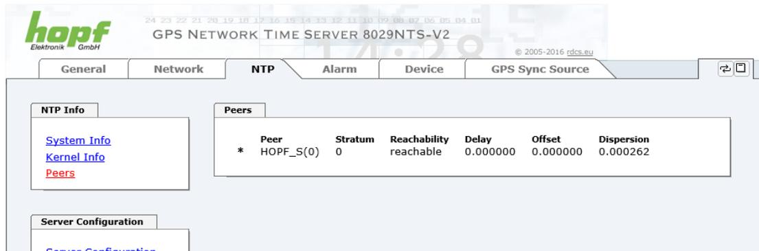
The screenshot shows the web interface for the hopf GPS Network Time Server. The 'NTP' tab is selected, displaying the following information:
