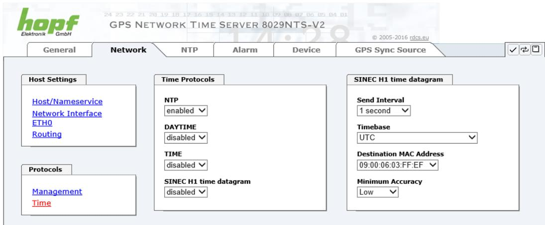
The screenshot shows the configuration page for the SINEC H1 time telegram. The page title is "GPS NETWORK TIME SERVER 8029NTS-V2". The "SINEC H1 time datagram" section is active, showing the following settings:
