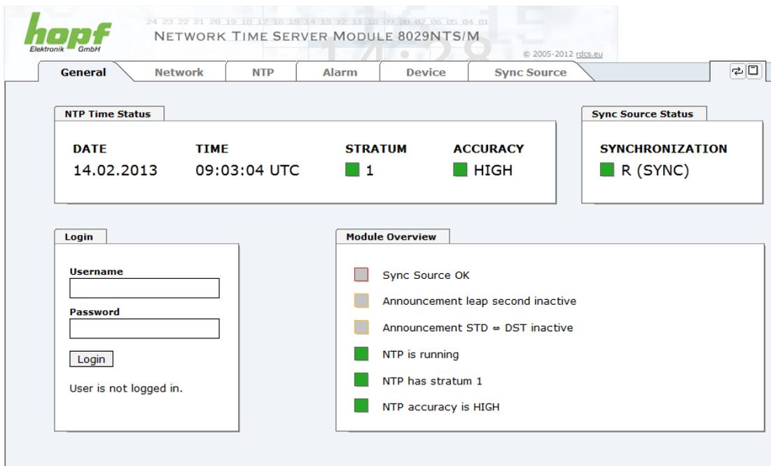
The screenshot displays the 'General' tab of the WebGUI for the 'NETWORK TIME SERVER MODULE 8029NTS/M'. The interface includes a navigation bar with tabs for 'General', 'Network', 'NTP', 'Alarm', 'Device', and 'Sync Source'. The main content area is divided into several sections:
