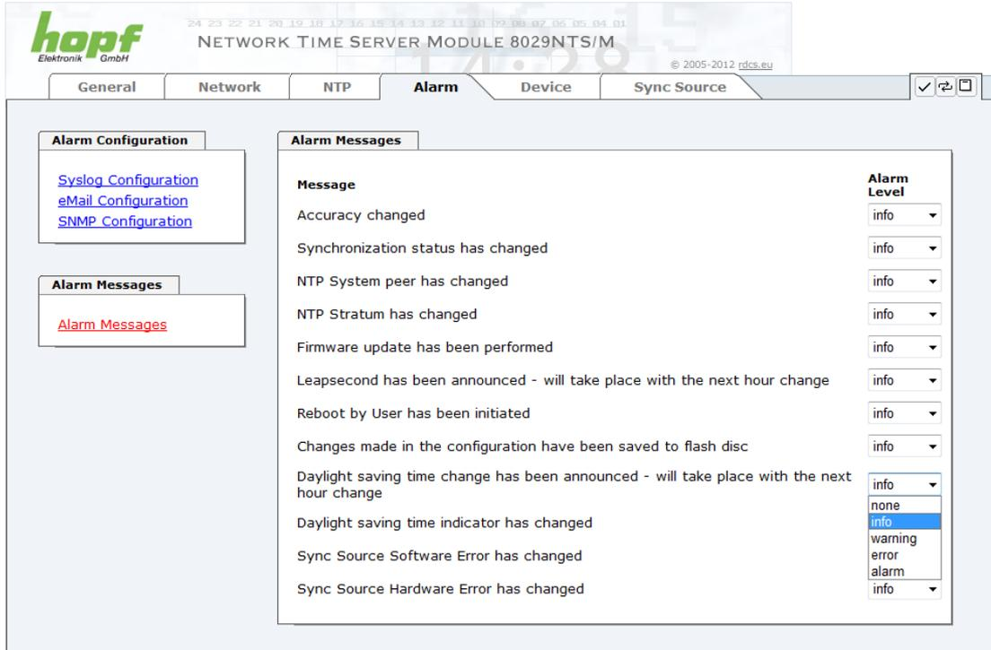
The screenshot shows the 'Alarm Messages' configuration page. On the left, there are links for 'Syslog Configuration', 'eMail Configuration', and 'SNMP Configuration'. Below these are 'Alarm Messages' and 'Alarm Messages' (highlighted in red). The main area lists various messages with their configured 'Alarm Level'.
