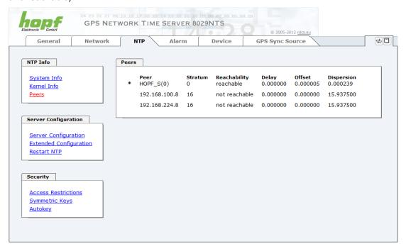
Three lines can be seen in the above image. The first line displays the **hopf** - refclock ntp driver that gets the time information directly from the Sync Source.
