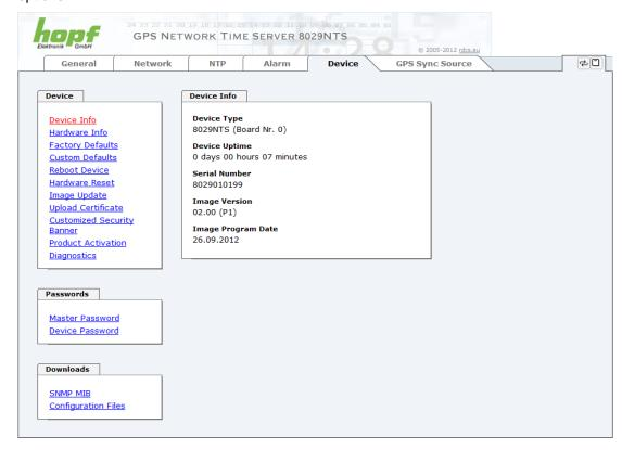
This tab provides the basic information about the hardware of Module 8029NTS as well as software/firmware. Password administration and the update services for the module are also made accessible via this website. The complete download zone is also a component of this site.
