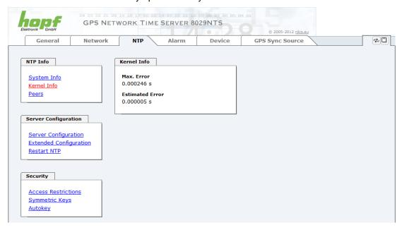
This screenshot shows a maximum kernel clock error of 0.246 msec (milliseconds). The estimated error value is 5 µs (microseconds).
