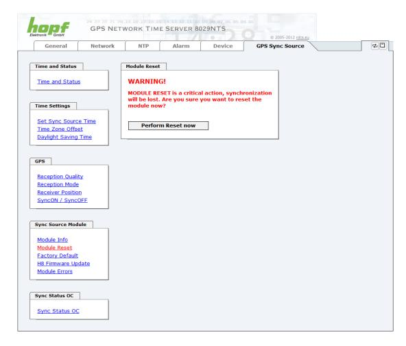
This function triggers a hardware reset of (just) the Sync Source (here Module 8021GPS).
