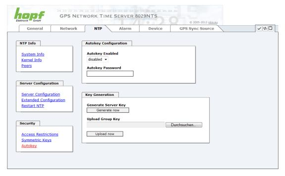
In order to enable Autokey v2 authentication, the "Autokey Enabled" option must be set to "enabled" and a password specified (may not be blank).
