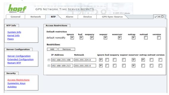
Restrictions are used in order to control access to the System's NTP service and these are regrettably the most misunderstood options of the NTP configuration.
