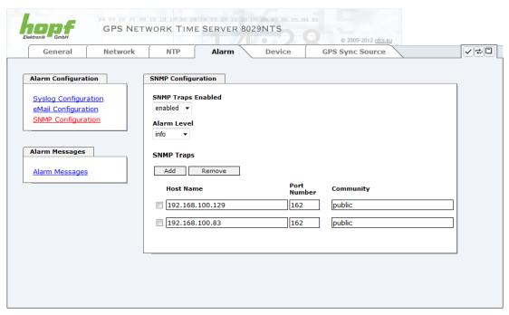
SNMP traps are sent to the configured hosts over the network. It should be noted that these are based on UDP and therefore it is not certain that they will reach the configured host!
