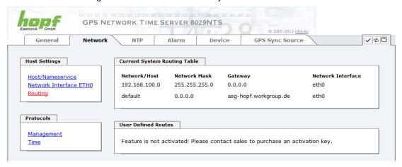
The gateway / gateway host need to be in the local sub-network range of the module in order to use the routes.
