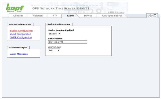
The alarm level designates the priority level of the messages to be transmitted and the level from which transmission should take place (see *Chapter 7.3.4.4 Alarm Messages*).
