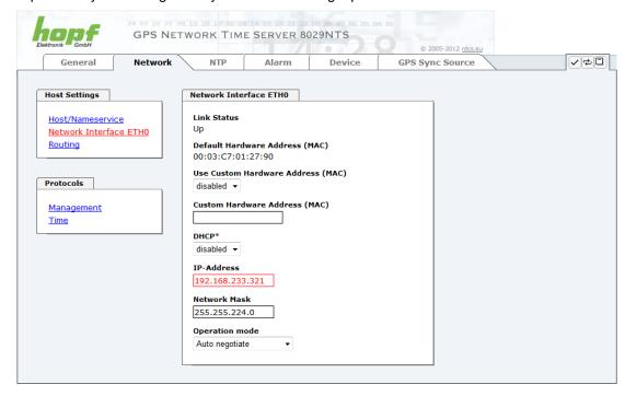
As illustrated in the above image, an invalid value (e.g. text where a number should be entered, IP address not within the range etc.) is identified by a red border when an attempt is made to accept these settings. It should be noted here that this is only a semantic check and not to test whether an entered IP address can be used on the own network or in the configuration! As long as an error message is displayed it is not possible to save the configuration in the flash memory.
