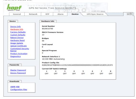
The display "Current DIP Switch Settings" is not applicable for this device.
