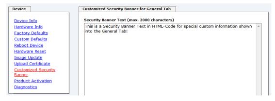
The security information can be written as 'unformatted' text as well as in HTML format. There are 2000 characters available to write failsafe into the Time Server 8029NTS/GPS.
