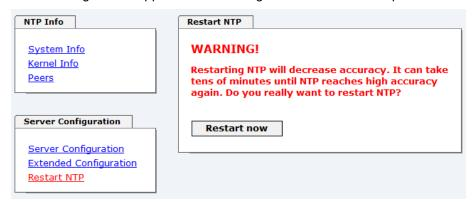
Restarting NTP services is the only possibility of making NTP changes effective without having to restart the entire Time Server 8029NTS/GPS. As can be seen from the warning message, the currently reachable stability and accuracy get lost caused by this restart.
