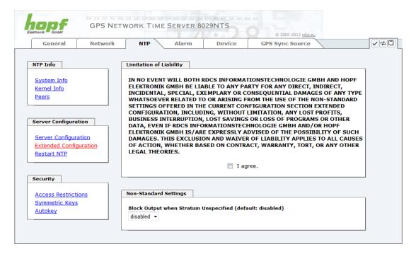
For activation of this special NTP setting, the customer's approval shown in the WebGUI needed to be declared by checking the field "I agree".
