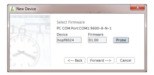
Probe connecting device 8024GPS. *Forward* confirms the selection.
