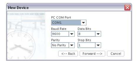
Configuration of computer's serial port with serial parameters (9600-8-N-1, like shown in the screenshot). Forward confirms the selection.
