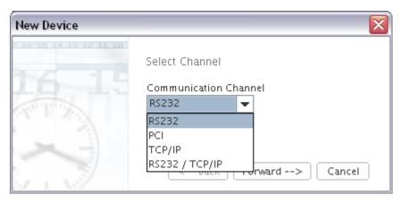
First, the Communication Channel to the device 8024GPS to be opened has to be defined as RS232. Forward confirms the selection.
