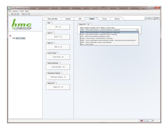
The synchronization status is represented from the bottom of the following table (INVA) up with increasing quality.
