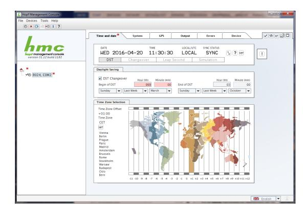
In case of an invalid input, a red asterisk \* will be shown and the causing input control is highlighted with pink background colour.
