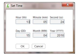
This dialog is initialized with the computer's current time. All values are changeable. After pushing the OK button, the time configuration values will be sent to the clock immediately.
