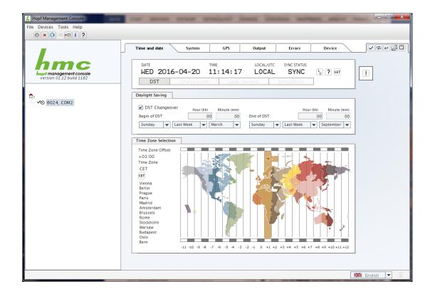
The configuration view is divided into functional tabs. Click on one of these tabs to navigate through the board. The selected tab is identified by a darker background colour, see the above image (tab "Time and date" in this case).
