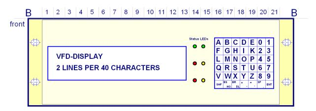
(here with option "BG7008/6LED" – front panel for system 7001RC including 6x status LED)
