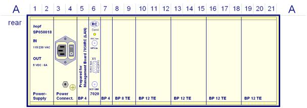
Up to 14 slots (including management board (LAN) 7050RC for system 7001RC) are available on a 3U rack for 'Function Boards' / 'RC-Function Boards' with 4HP faceplate width. Where 'Function Boards' or 'RC-Function Boards' with 8, 12 or 16HP width are used, the number of slots is reduced accordingly.
