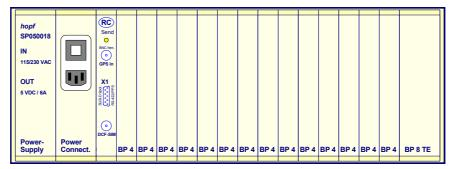
Up to 14 slots are available on a 3U rack for 'Function Boards' / 'RC-Function Boards' with 4HP faceplate width. Where 'Function Boards' or 'RC-Function Boards' with 8, 12 or 16HP width are used, the number of slots is reduced accordingly.
