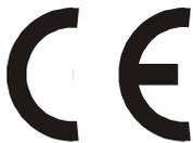
This device fulfils the requirements of the EU directive 89/336/EWG "Electromagnetic compatibility" and 73/23/EWG "Low voltage equipment".
