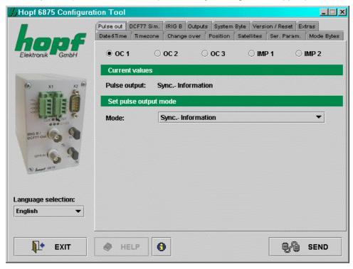
The current values for the selected output or pulse are requested and displayed. Depending on the **"Modus"** which has been set additional methods of configuration will appear or fade. The following modes are supported:
