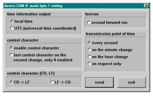
You find the set-function for the **mode byte 1** by selecting the menu **"communication"** and **"mode byte 1"**. The mode byte 1 dialog for the selected device appears which shows the actual settings of the clock. You can configure the output system to your specifications. Start the transmission with the **"send"** button. When the data have been accepted a dialog window appears with the following information
