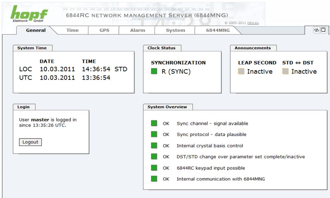
The screenshot shows the Hopf WebGUI interface for a 6844RC NETWORK MANAGEMENT SERVER (6844MNG). The interface includes a navigation bar with tabs for General, Time, GPS, Alarm, System, and 6844MNG. The main content area is divided into several sections:
