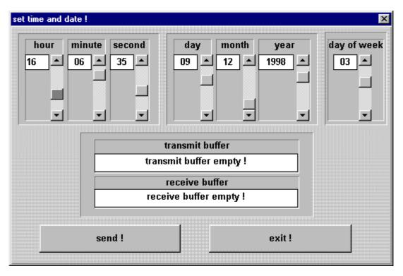
You can change the time by moving the scroll bar next to the displays. After setting the correct time, start the transmission to the clock with the **"send"** switch. In the status field **"transmit buffer"** the data string which was transmitted to the clock appears. When the transmission is successful the same data string is shown in the **"receive buffer"**
