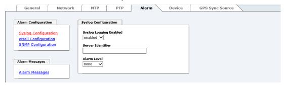
The alarm level designates the priority level of the messages to be transmitted and the level from which transmission should take place (see *Chapter 7.3.5.4 Alarm Messages*).
