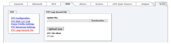
In case of announcing a leap second by the synchronization source the leap second file will automatically be updated.
