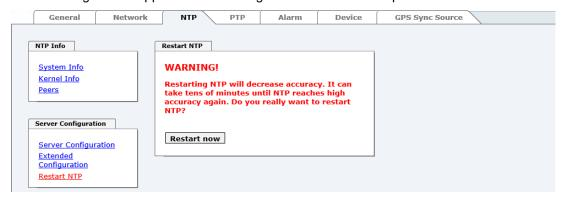
Restarting NTP services is the only possibility of making NTP changes effective without having to restart the entire Time Server 8030NTS/GPS. As can be seen from the warning message, the currently reachable stability and accuracy get lost caused by this restart.
