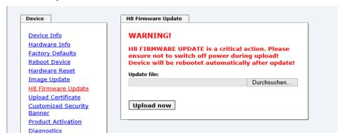
A restart of the device with the new Firmware is done automatically after the H8-Firmware update.
