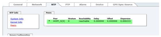
The first line displays the *hopf* - refclock ntp driver that gets the time information directly from the Sync Source.
