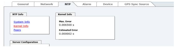
This screenshot shows a maximum kernel clock error of 6.500 msec (milliseconds). The estimated error value is 2 µs (microseconds).
