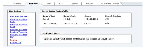
The gateway / gateway host need to be in the local sub-network range of the module in order to use the routes.
