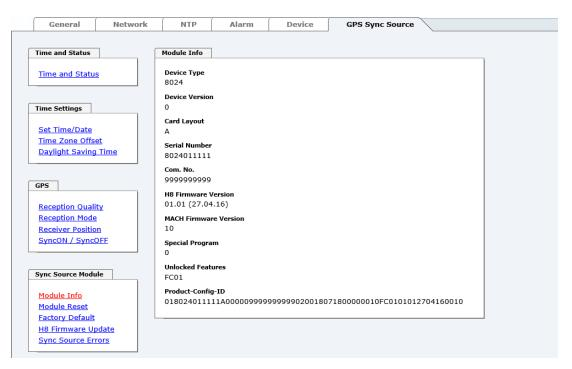
This tab indicates information about the hardware and software of the Module 8024GPS (Sync Source) implemented in the Time Server 8029NTS/GPS.
