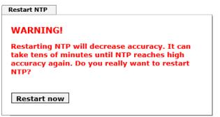
Restarting NTP services is the only possibility of making NTP changes effective without having to restart the entire Time Server 8029NTS/GPS. As can be seen from the warning message, the currently reachable stability and accuracy get lost caused by this restart.
