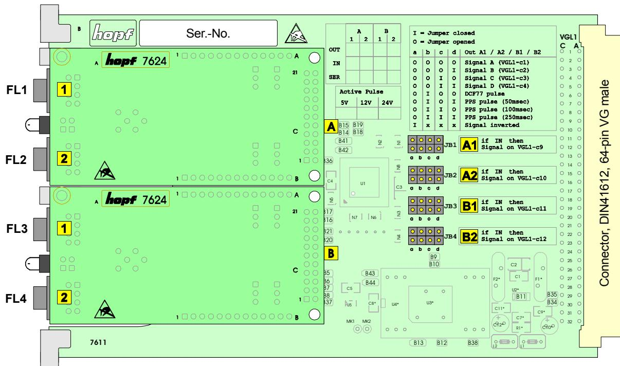
**FL1-FL4: FO-Transmitter and Receiver designed as ST**
