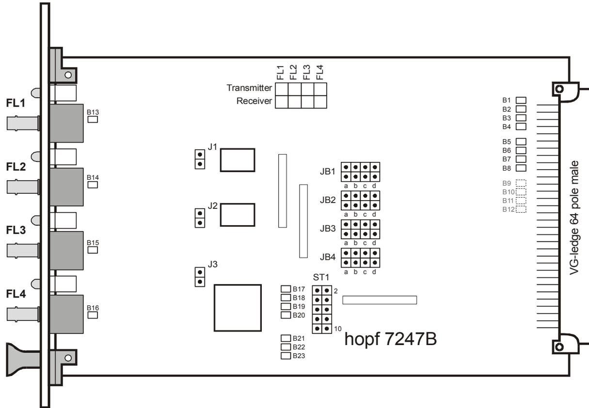
**FL1-FL4: FO-Transmitter and Receiver designed as ST (LWL-Sender und -Empfänger in Bauform ST)**
