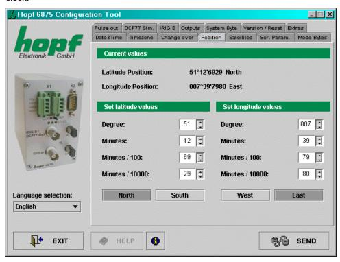
Setting the approximate location position (if known) shortens the time required for first initialisation of the GPS receiver in the radio-controlled clock.
