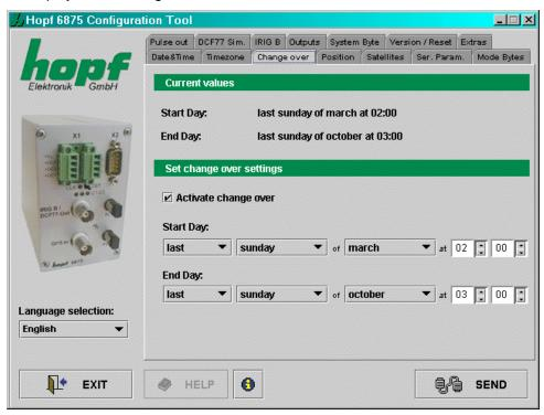
In order to set the changeover times the changeover function must first be activated. If no changeover is required this must be deactivated  $\Rightarrow$  time of day (local time) then runs in standard time status.
