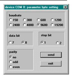
You find the setting for baud rate, data bit, stop bit and parity by selecting the menu "communication" and "serial parameter". The parameter dialog for the selected device appears.
