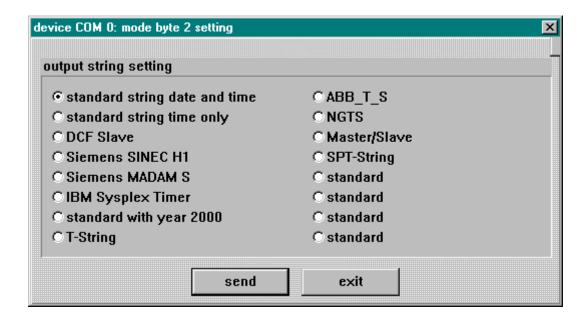
Click at the according checkbox for the data string you want and start the transmission to the clock with the **[send]** switch. When the data has been accepted a dialog window appears with the information:
