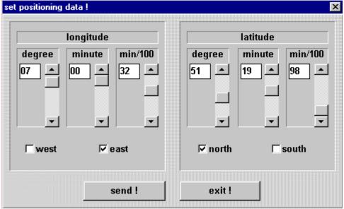
After entering the data use the "send" switch to start the transmission to the clock. If the transmission was successful a pop-up window appears with the message "new values are stored in clock device".
