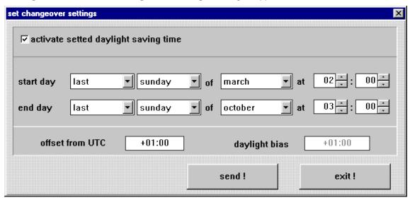
Before activating the dialogue the current settings are read from the clock and displayed in the editing field. Here the points of time are entered when during the course of a year the time is to changeover to either daylight saving time or standard time on location.
