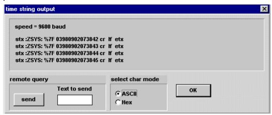
The presently set baud rate is shown in the line "speed = 9600 baud".
