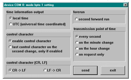
You find the set-function for the **mode byte 1** by selecting the menu **"communication"** and **"mode byte 1"**. The mode byte 1 dialog for the selected device appears which shows the actual settings of the clock. You can configure the output system to your specifications. Start the transmission with the **"send"** button. When the data have been accepted a dialog window appears with the following information
