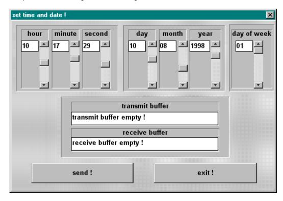
You can change the time by moving the scroll bar next to the displays. After setting the correct time, start the transmission to the clock with the "send" switch. In the status field "transmit buffer" the data string which was transmitted to the clock appears. When the transmission is successful the same data string is shown in the "receive buffer".
