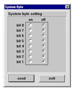
This function serves to switch on/off different internal program functions. Only bit 1-5 have a function at present. You find the "system byte" dialog under the "set" menu. After the selection the shown dialog box is displayed with the actual settings.
