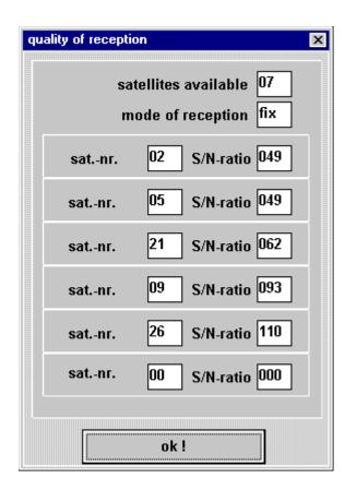
"Satellites available" lists the number of satellites visible in this antenna position in this location. The field "mode of reception" shows the actual selected mode.
