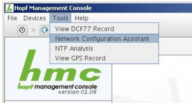
After a successful start of the ***hmc* Network Configuration Assistant** and completed search of the **hopf** LAN Modules, the configuration of the base LAN parameters can be done.
