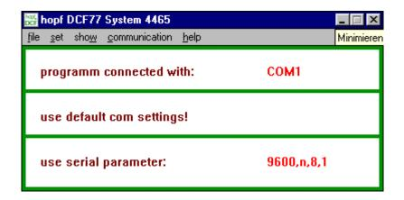
The software automatically finds the <u>first</u> free COM-port and shows the connection by clicking on "**programm connected with"** in the main window of the application. Also the actual parameters for the serial communication and the possible used file is displayed.
