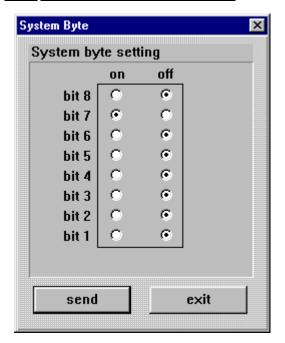
This function is used to switch internal programme functions on and off. You'll find the settings of the system byte under the menu item "set" and the entry "system byte". The "System byte" dialogue appears showing the present bit positions in the clock.
