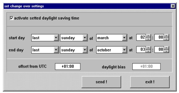
Before activating the dialogue the current settings are read from the clock and displayed in the editing field. After setting the mark in the field 'active settled daylight saving time' the points of time are entered here when during the course of the year daylight saving- or standard time for this location are changed over. Hours and month are entered separately for start of daylight saving time (summer time) and start of standard time (winter time).
