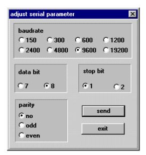
Confirm your entry by pressing the **"send"** key. The new parameters are taken over into the clock. When the data are taken over the following information is shown in the dialogue window:
