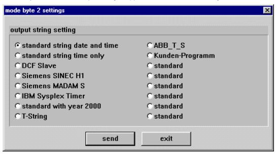
Click at the according checkbox for the data string you want and start the transmission to the clock with the "send" switch. When the data have been accepted a dialogue window appears with the information:
