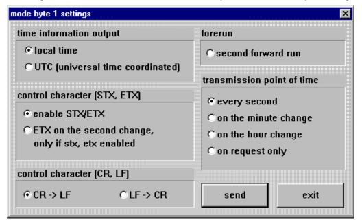
You find the set-function for the **"mode byte 1"** by selecting the menu **"communication"** and **"mode byte 1"**. The mode byte dialogue appears with the current settings in the clock.
