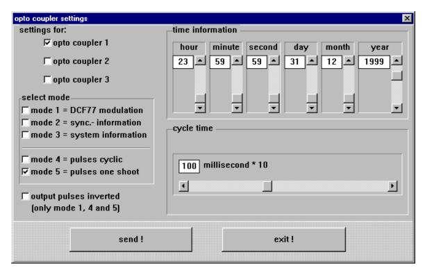
The different functions are called modes and selected in the group window "select mode". Only one setting each can be selected. Depending on the selected function (mode), either the time information in the group window "time information" or the value for the pulse width can be set in the window "cycle time".
