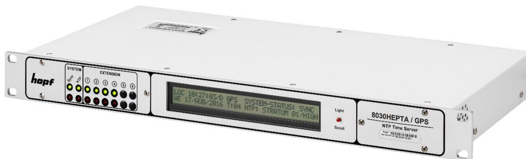
front view 8030HEPTA-02 with at-a-glance status-LEDs and LCD Display
