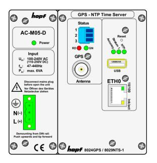
The Time Server is integrated into a compact DIN Rail housing and is characterized by its easy and simple operation, although it offers a **broad range of functions**. Some of the practice-oriented functionalities are:
