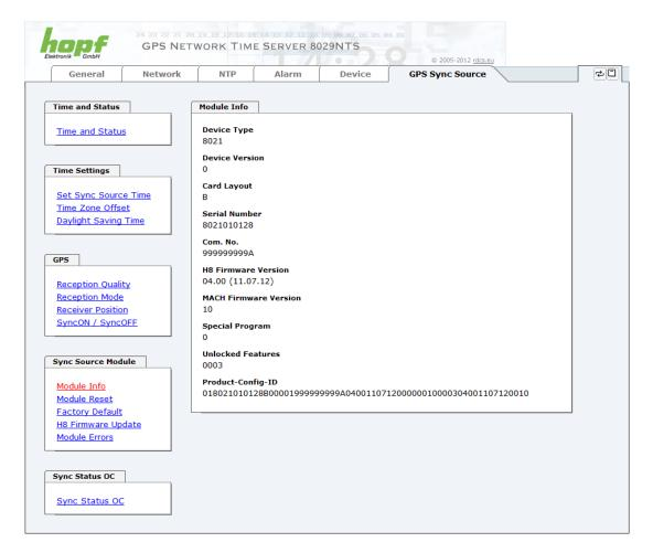
This tab indicates information about the hardware and software of the Module 8021GPS (Sync Source) implemented in the Time Server 8029NTS/GPS.
