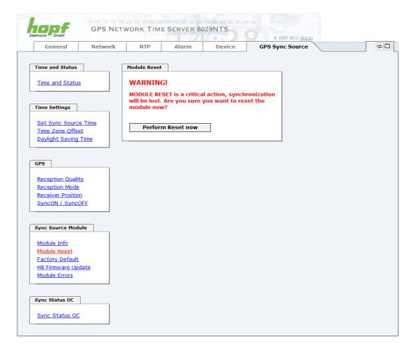
This function triggers a hardware reset of (just) the Sync Source (here 8021GPS).
