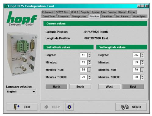
Setting the position is only necessary when commissioning. This shortens the time required for first initialisation of the GPS receiver in the radio-controlled clock.
