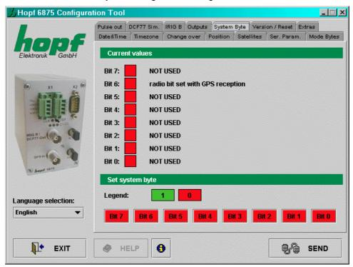
Each bit has two possible statuses: 1 (function activated) and 0 (function deactivated).
