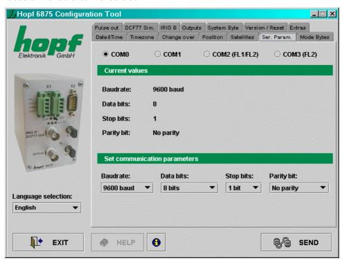
The selection of the interface to be configured is made in the upper part of the frame by clicking the appropriate interface [COM0, COM1, COM2 (FL1/FL2) und COM3 (FL2)]. The current values for the selected interface are requested and displayed. These values can be changed by selecting from the lists intended for this purpose.
