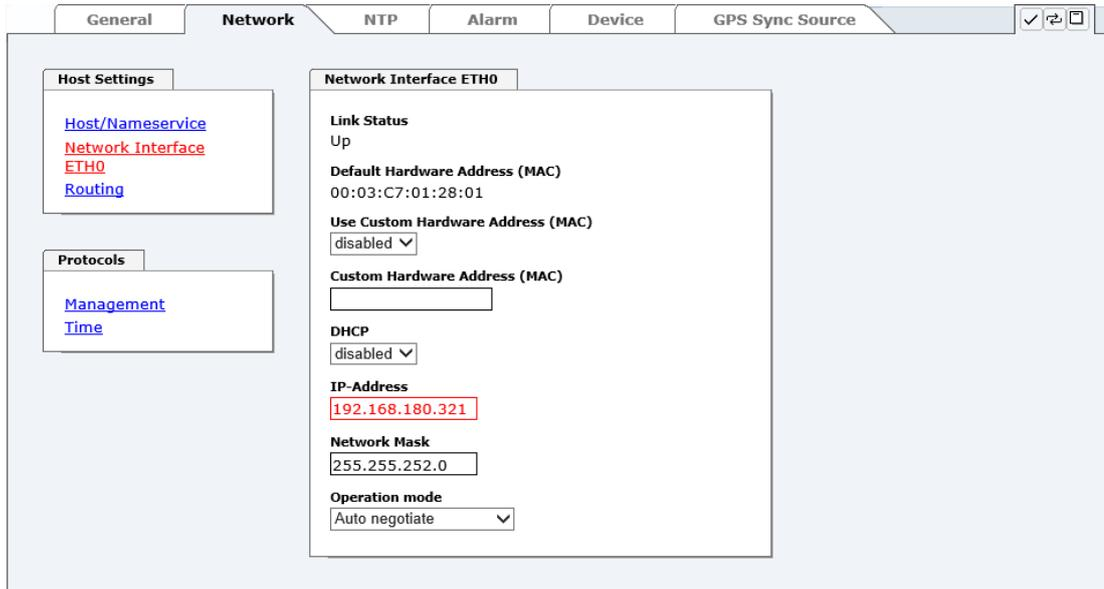
The screenshot shows the 'Network Interface ETH0' configuration page. The 'IP-Address' field contains the value '192.168.180.321', which is highlighted with a red border, indicating a validation error. Other fields include 'Link Status' (Up), 'Default Hardware Address (MAC)' (00:03:C7:01:28:01), 'Use Custom Hardware Address (MAC)' (disabled), 'Custom Hardware Address (MAC)' (empty), 'DHCP' (disabled), 'Network Mask' (255.255.252.0), and 'Operation mode' (Auto negotiate).
