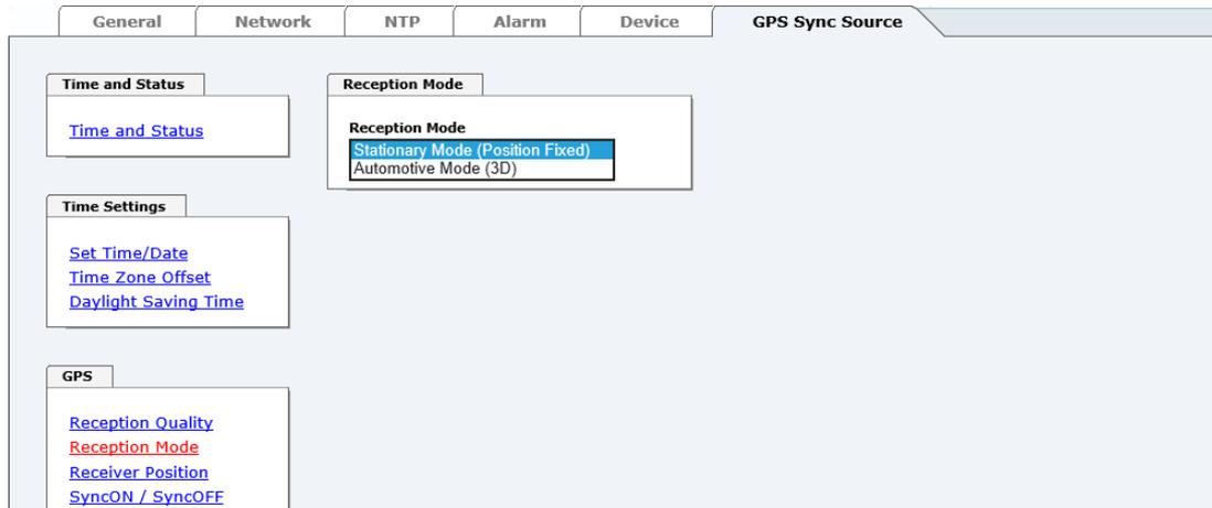
The screenshot shows the 'GPS Sync Source' configuration page with the 'Reception Mode' dropdown menu open. The menu options are 'Stationary Mode (Position Fixed)' and 'Automotive Mode (3D)'. The 'Stationary Mode (Position Fixed)' option is currently selected.
