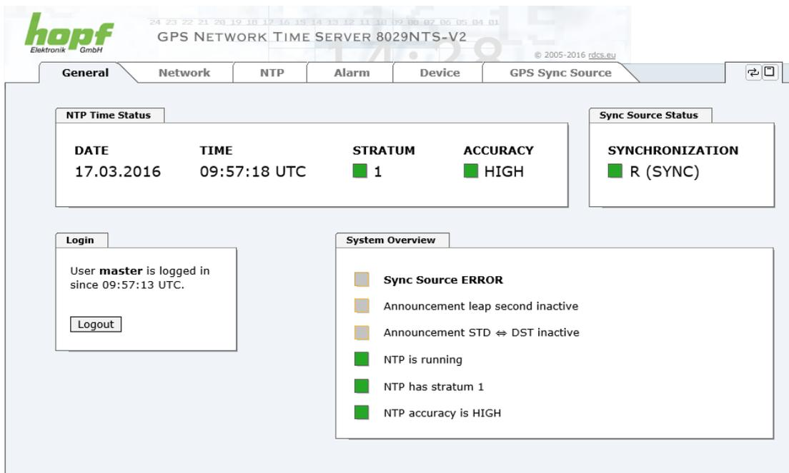
The screenshot shows the 'General' tab of the hopf WebGUI. At the top, there is a navigation bar with tabs for 'General', 'Network', 'NTP', 'Alarm', 'Device', and 'GPS Sync Source'. The main content area is divided into several sections:
