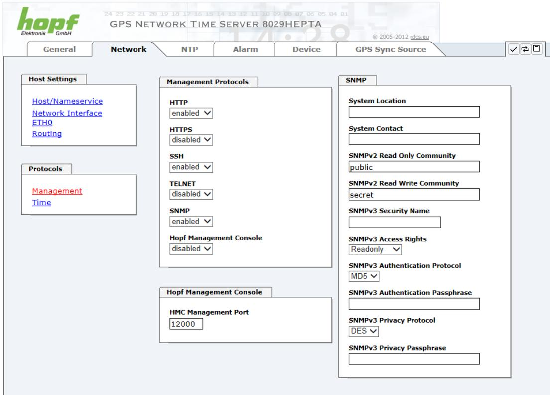
The screenshot shows the configuration interface for a Hopf device. The top navigation bar includes tabs for General, Network, NTP, Alarm, Device, and GPS Sync Source. The 'Network' tab is active. The interface is divided into several sections:
