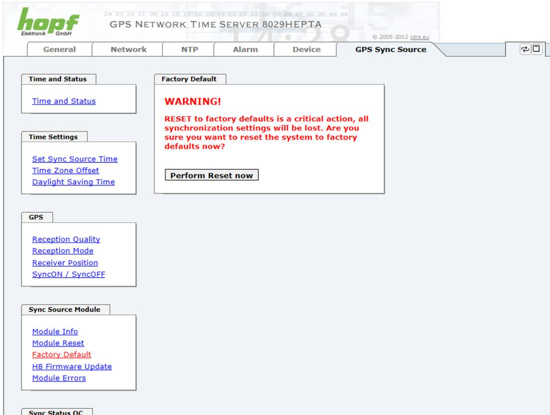
The screenshot shows the web interface for the 'GPS NETWORK TIME SERVER 8029HEPTA'. The 'GPS Sync Source' tab is active. A prominent warning box is displayed, stating: **WARNING!** RESET to factory defaults is a critical action, all synchronization settings will be lost. Are you sure you want to reset the system to factory defaults now? Below the warning is a button labeled 'Perform Reset now'. Other visible sections include 'Time and Status', 'Time Settings', 'GPS', and 'Sync Source Module'.
