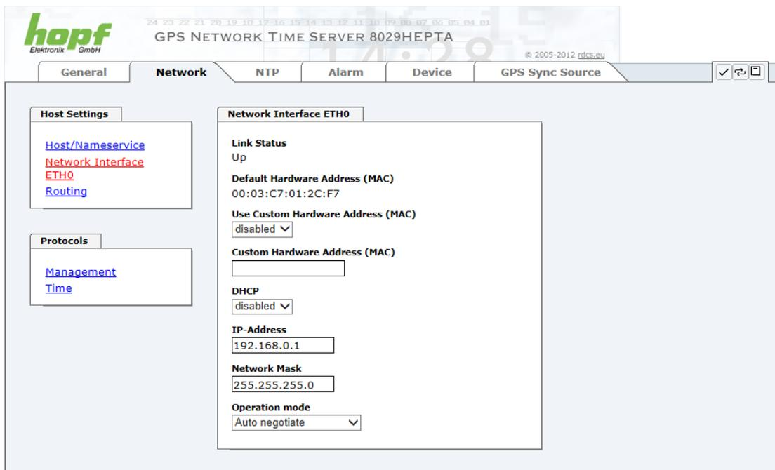
The screenshot displays the configuration interface for the Network Interface ETH0. The top navigation bar includes tabs for General, Network, NTP, Alarm, Device, and GPS Sync Source. The main content area is divided into two sections: Host Settings and Network Interface ETH0. The Host Settings section contains links for Host/Nameservice, Network Interface, ETH0, and Routing. The Network Interface ETH0 section contains the following settings:
