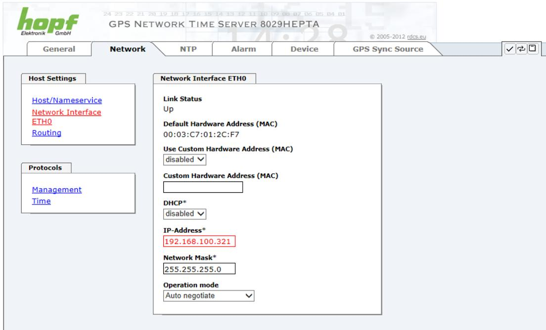
The screenshot shows the 'Network' configuration page for 'Network Interface ETH0'. The 'IP-Address\*' field contains the value '192.168.100.321', which is highlighted with a red border, indicating a semantic error. Other fields include 'Link Status' (Up), 'Default Hardware Address (MAC)' (00:03:C7:01:2C:F7), 'Use Custom Hardware Address (MAC)' (disabled), 'Custom Hardware Address (MAC)' (empty), 'DHCP\*' (disabled), 'Network Mask\*' (255.255.255.0), and 'Operation mode' (Auto negotiate).
