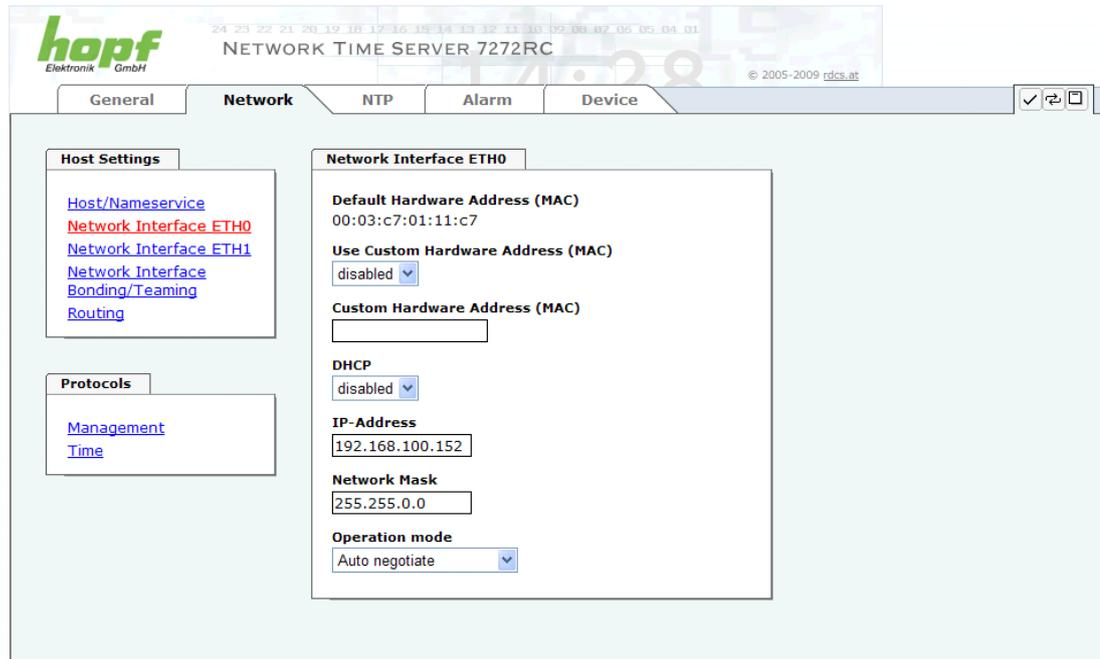
The screenshot shows the configuration page for Network Interface ETH0. The top navigation bar includes 'General', 'Network', 'NTP', 'Alarm', and 'Device'. The 'Network' tab is active. On the left, there are links for 'Host/Nameservice', 'Network Interface ETH0', 'Network Interface ETH1', 'Network Interface', 'Bonding/Teaming', and 'Routing'. Below these are 'Protocols' with links for 'Management' and 'Time'. The main configuration area for 'Network Interface ETH0' includes:
