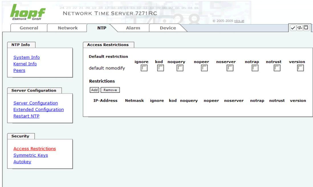
The screenshot shows the web interface for the hopf Network Time Server 7271RC. The main navigation tabs are General, Network, NTP, Alarm, and Device. The NTP tab is selected, showing several sub-sections:
