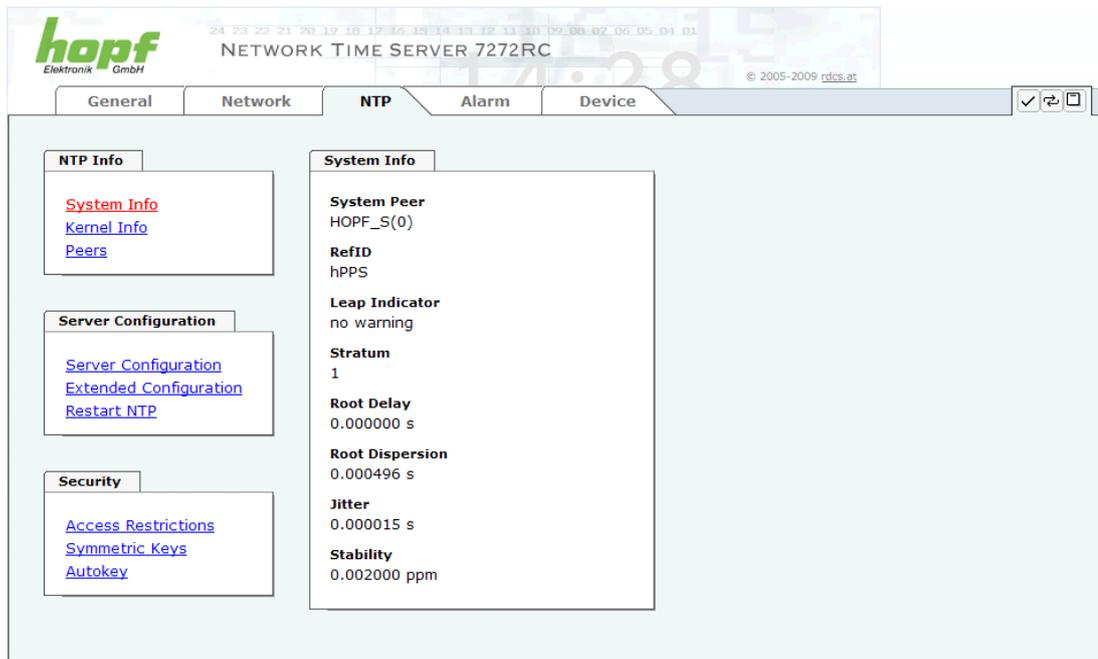
The screenshot displays the web interface for a Network Time Server (NTP) configuration. The top navigation bar includes tabs for General, Network, NTP (selected), Alarm, and Device. The main content area is divided into three sections: NTP Info, Server Configuration, and Security. The NTP Info section is further divided into System Info and System Peer. The System Info section displays the following data:
