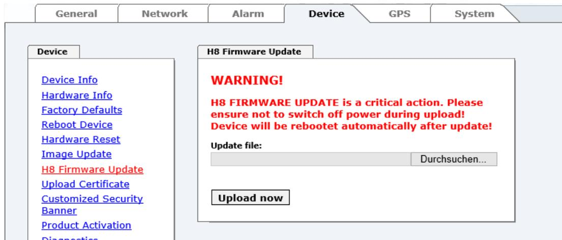
A restart of the Board with the new Firmware is done automatically after the H8-Firmware update.
