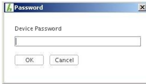
Device Password **<device>** is set for LAN boards 7052RC on delivery. So no further entry is required here – click on the button **OK** to confirm.
